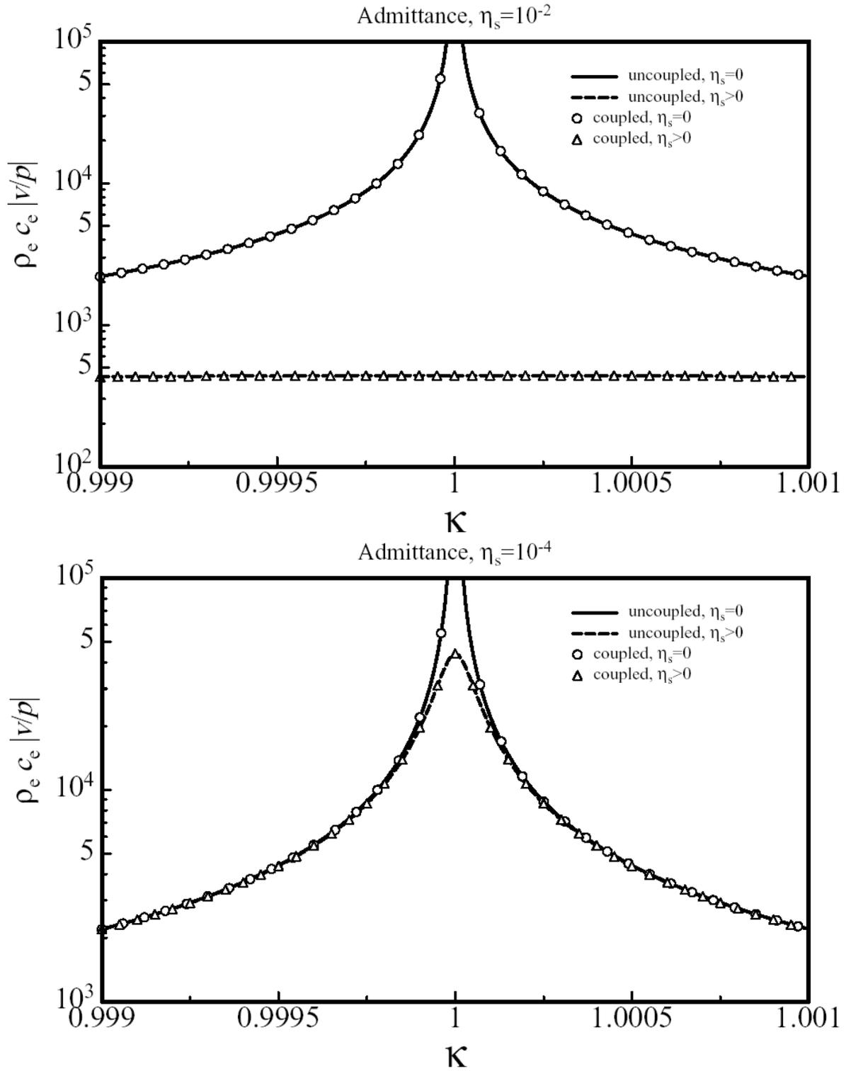
Abb. 4: Dimensionless admittance  $\rho_e c_e |v(\omega)/p_i|$  of sphere in water  $\rho_e/\rho_s = 0.127$ , variation of the structural loss factor.
