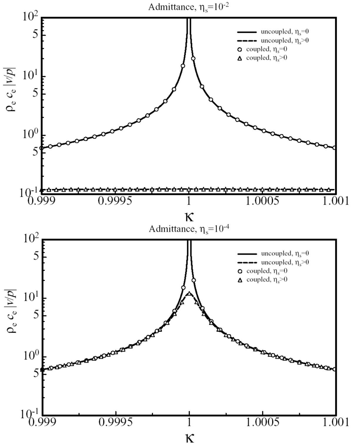
Abb. 3: Dimensionless admittance  $\rho_e c_e |v(\omega)/p_i|$  of sphere in air  $\rho_e/\rho_s = 1.5 \cdot 10^{-4}$ , variation of the structural loss factor.
