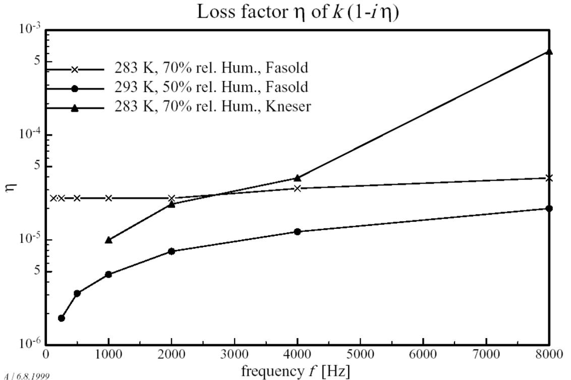
Abb. 2: Loss factor of frequency  $f = \Omega/(2\pi)$  in air.
